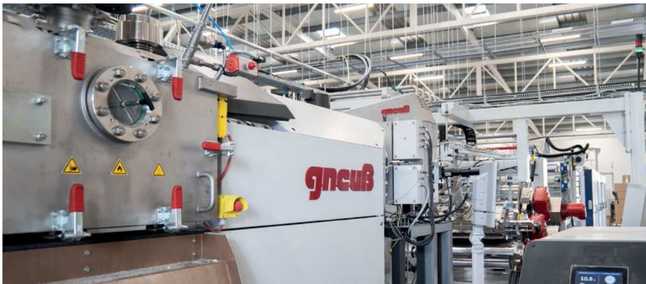
Gneuss OMNI extrusion line with MRS extruder and RSFgenius melt filtration system
