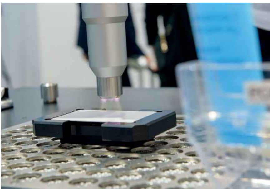
Plasma activation of plastic surfaces for improved adhesion properties
