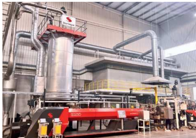
Starlinger's recoSTAR PET art bottle-to-bottle recycling system produces up to 3,000 kg food-grade rPET per hour (© Novatex)
