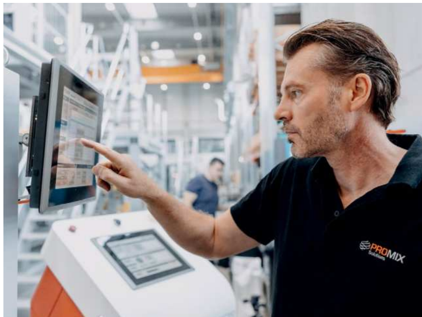
The "Visco P" inline viscometer is now available with a complete control loop and, when combined with a dosing unit, enables the control of an additive based on the viscosity measured during the production process
